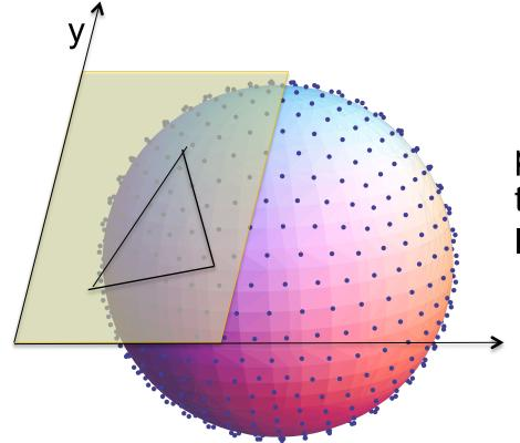
project spherical triangle onto local tangent plane
