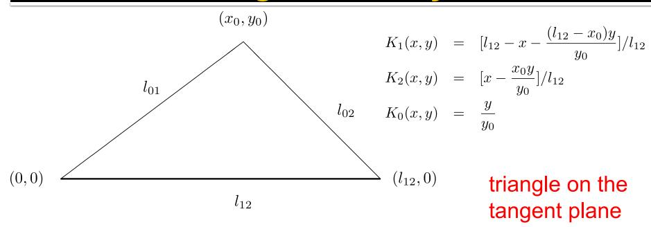
On each triangle expand:  $\phi(x,y) = \sum_{i} K_i(x,y)\phi_i$  an integrate
