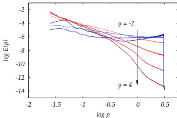
Transition roughly at  $y \simeq 3$  – high-momentum modes effectively decouple from forcing mechanism
