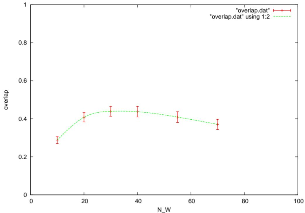
Wuppertal smearing with  $\alpha = 3$ ,  $N = 35$  using APE-smeared ( $A = 2.85$ ,  $N = 25$ ) gauge links.
